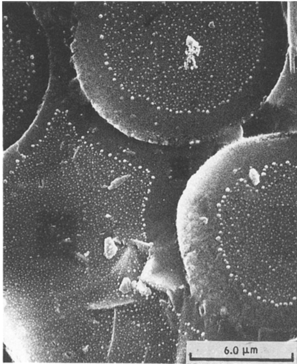
Figure 4 Scanning electron micrograph of a Duran glass/SiC composite produced with a titanium alkoxide solution.
